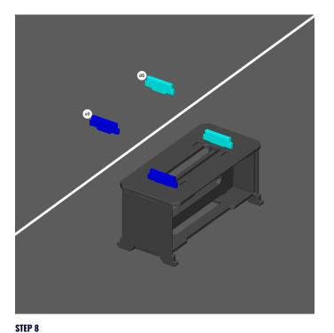
Glue the short rail pieces first, onto the bottom of the container assembly.
