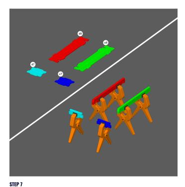
Fold, glue, and clamp as shown to create the bottom container rails.
